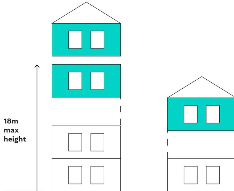
Class AD permits new flats on terrace dwellings as shown in Figure 18. Two-storeys and above can increase up to two-storeys and single-storeys can increase by an additional storey. There is an overall height limit of 18 metres.
