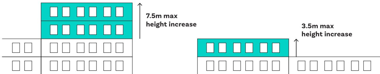
The highest part of the new roof compared to the existing building cannot exceed 3.5 metres for a single-storey building or 7.5 metres for a two-storey building and above.
