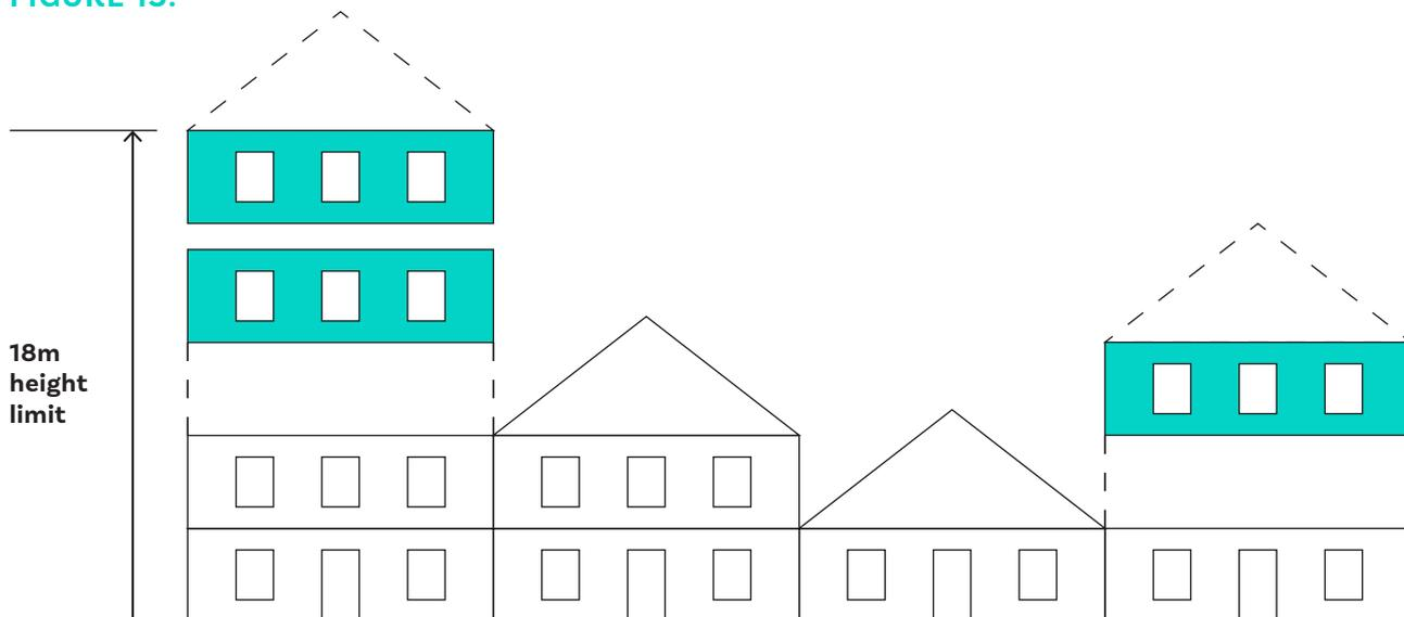
Class AC permits new flats on terrace dwellings as shown in Figure 15. Buildings two-storeys and above can increase by two-storeys, whereas one-storey buildings can increase by an additional floor. There is an overall height limit of 18 metres.
